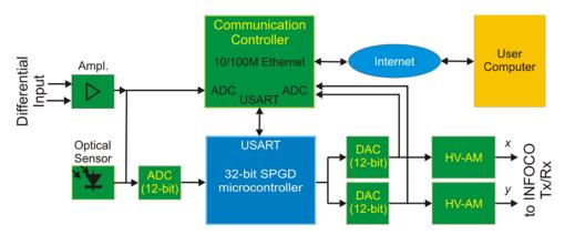
The INFOCO CU is an intelligent controller based on the latest microprocessor technology. The INFOCO CU receives either an optical or electrical input signal that is sent into a 12-bit analog-to-digital converter (ADC) and further to the 32-bit microcontroller running the proprietary advanced stochastic parallel gradient descent (SPGD<sup>+</sup>) control algorithm.
