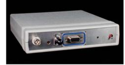
output signals of the low-voltage amplifiers with amplitude range  $\pm 2.5$  V or the output signals of the high-voltage amplifiers with amplitude range  $\pm 70$  V provide controls that are supplied to the INFOCO Tx or Rx. In addition, a communication controller provides the interface through a local area network (LAN) between the user's computer and the INFOCO CU, sending and receiving commands and system data.
