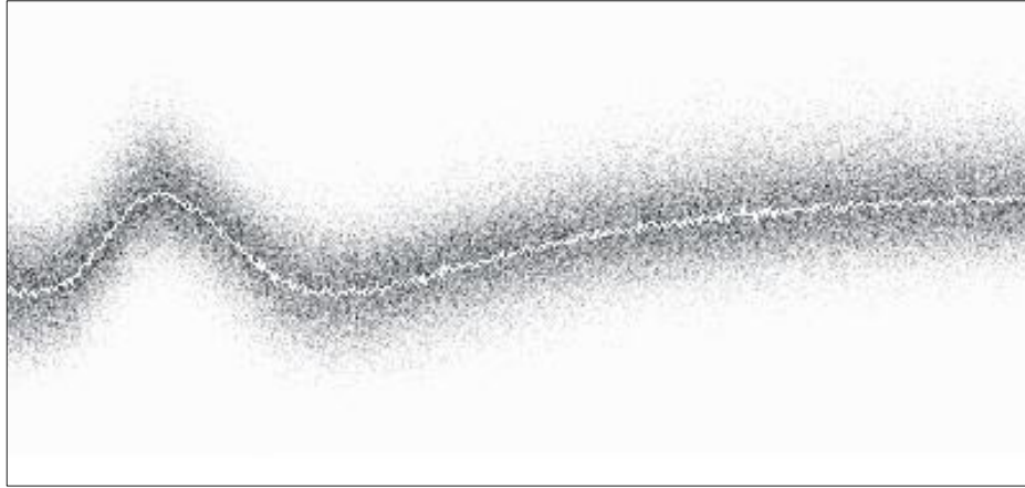
Figure 4: The distribution of output intensity responses to input voltages. The vertical axis of the picture is detected output intensity. The third axis (gray level of the points in the picture) is the number of occurrences of each input voltage output intensity pair.
